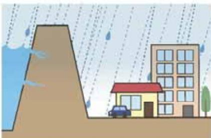
When river water increases during heavy rain, water pressure is applied to riverbanks.
